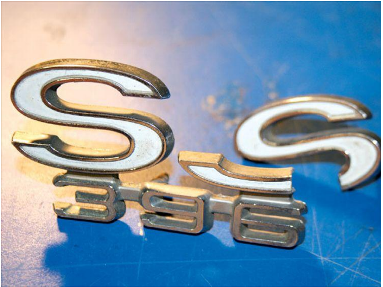
The SS396 emblem we re-created in cast plastic was cleaned and the painted inner portions sanded with 500-grit paper
