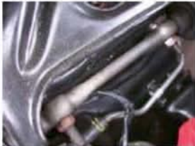
On many muscle-era GM and Ford vehicles, alignment adjustments are made with shims placed
