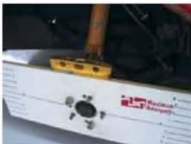
With the brake caliper and bracket removed, attach the gauge board to the hub with a couple
