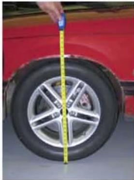
Begin by measuring the height of the hub above the floor at ride height. You'll need this
