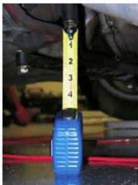
Weight is jacked around the car by adjusting the ride height at each corner. It's better to
