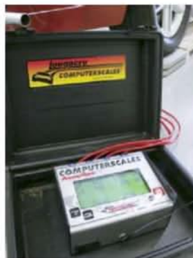
The digital readout on our Longacre Accuset computer scales displays individual corner weight
