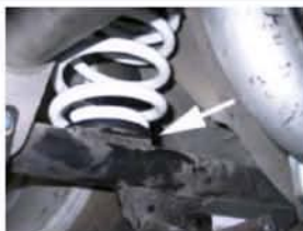
We raised the ride height of our Mustang's left-rear corner by 1/2 inch using a pair of polyurethane spring isolators (arrow), which is about the maximum change you'd like to make at any corner.
