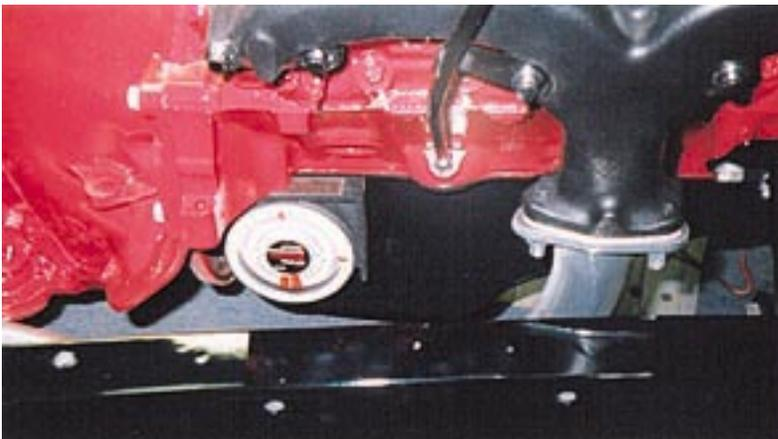
The engine/transmission should be set in the chassis with the rear approximately 3 degrees *below* horizontal. A magnetic-based protractor (shown) can be used to check the angle on the block where the starter mounts (or on the starter housing itself). Since the engine/trans mounts rarely are adjustable, the rear end housing will be adjusted to set the pinion angle. (See Figure 2.)
