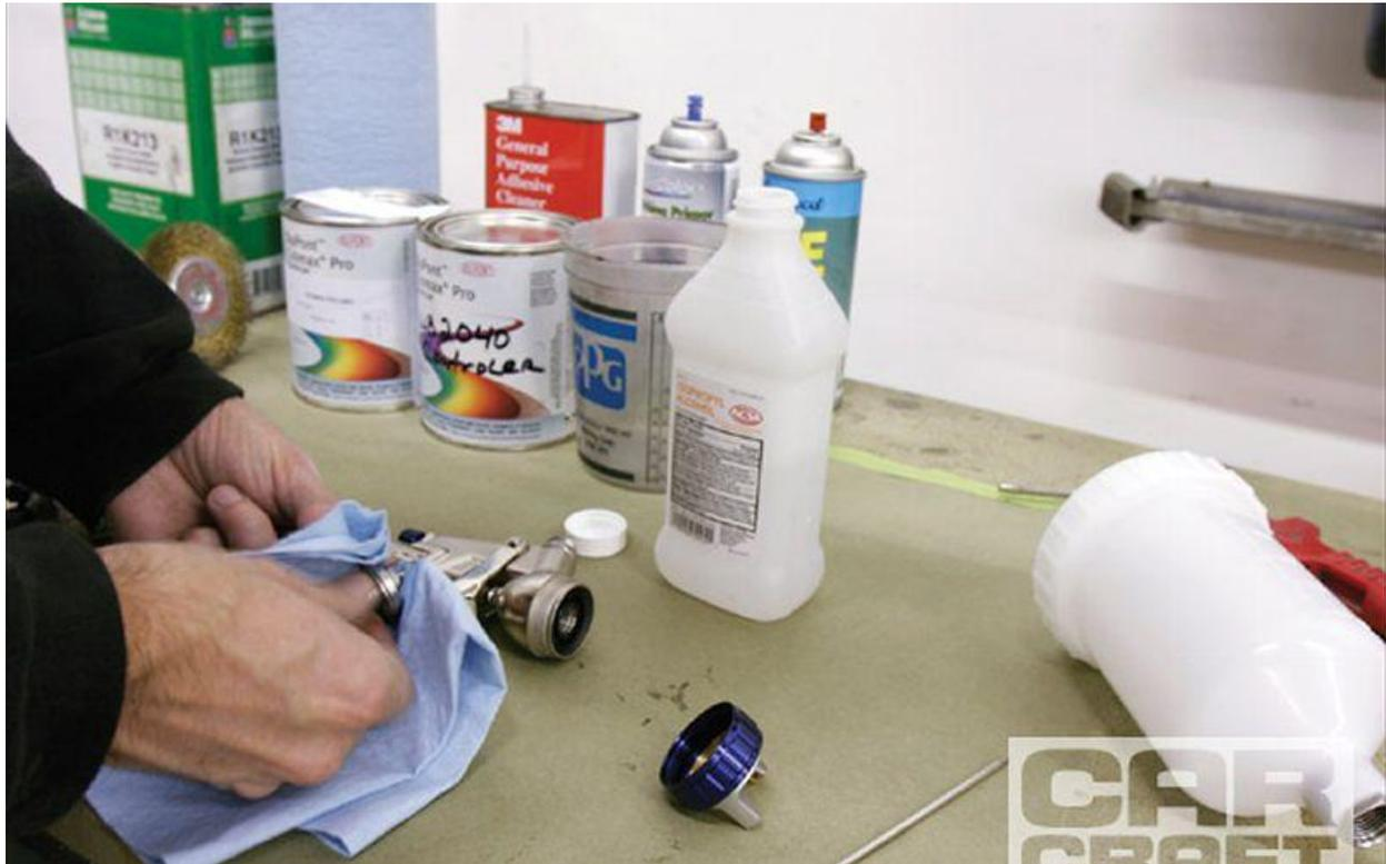
Avoid the temptation to use regular lacquer thinner to clean the gun. It does not react well to waterborne paint and causes the paint to clump up rather than thin out. Guess how we know that. Clogs are the last thing you want forming in your spray gun, so we cleaned everything with rubbing alcohol. Special surface-prep cleaners are made to go with waterborne paints. Be sure to buy some when you're buying the paint.
