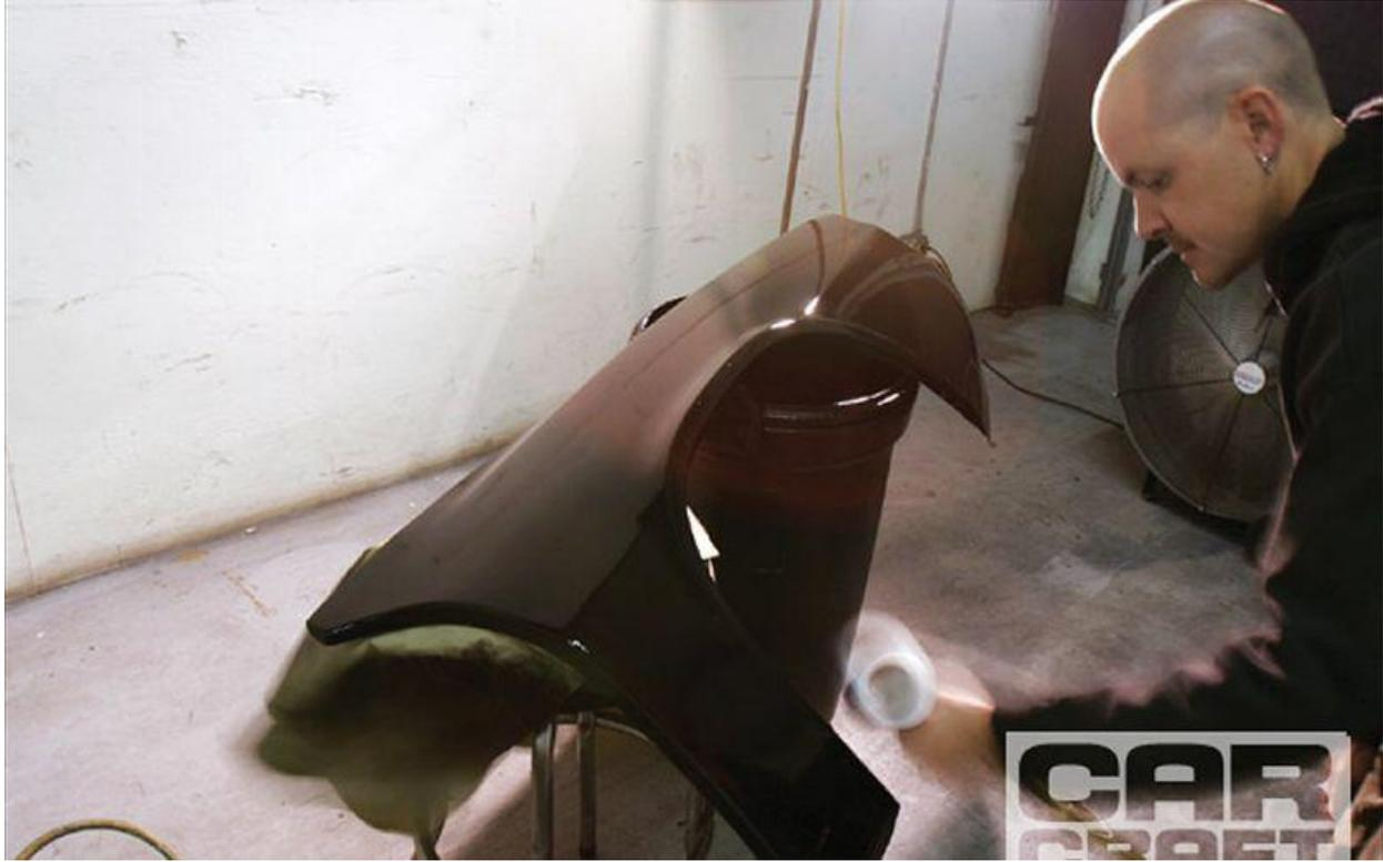
Once you're done spraying, turn on your fans and heaters. You can also buy handheld blowers that plug into your shop's air supply. If using a handheld one, hold it at a 45-degree angle to the panel. Always direct airflow across the panel. If you point straight at it, you can cause the paint to run.
