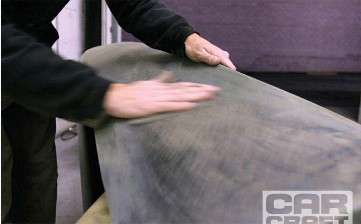
After spraying the recommended four coats of primer and waiting 30 minutes, we scuffed the whole panel with 320-grit sandpaper.
