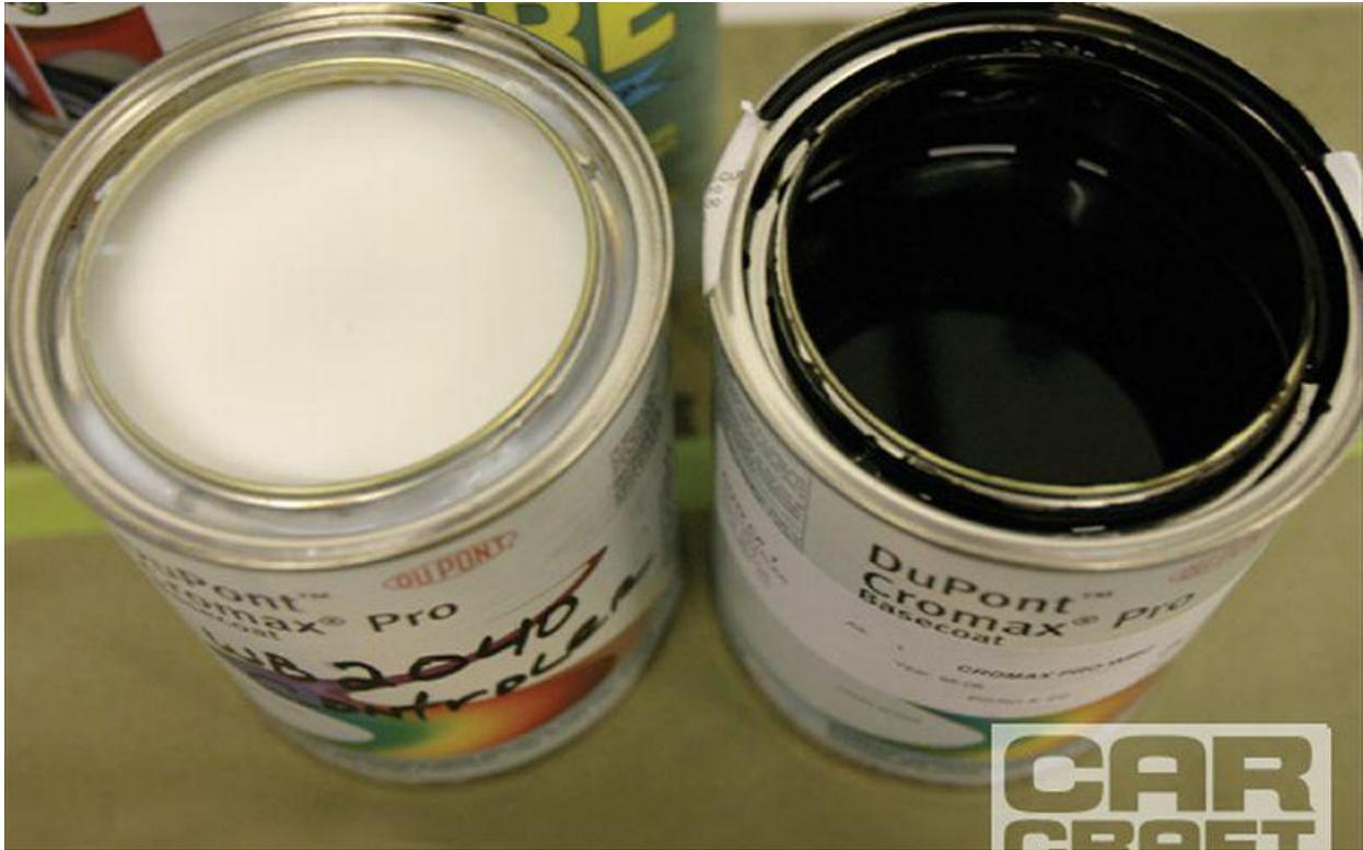
We bought a quart of DuPont CroMax in PX8, a Chrysler black, from Annex Autobody Supply in Los Angeles. Note that waterborne paints will usually come in a plastic container instead of steel. Because we bought such a small amount, our supplier just used a regular steel can. The white stuff is called the controller and takes the place of activator and thinner in regular solvent paint.
