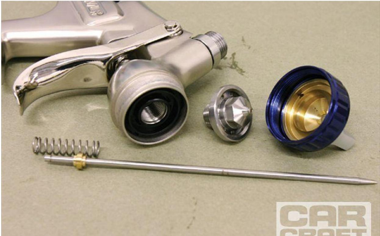
While there still is a little solvent in waterborne paint, there is a lot of water, so you need to use a paint gun designed to spray waterborne paint. The gun must have stainless innards that will not rust or corrode. We used Eastwood's new Concours HVLP gun and were pleased with its quality material and design, awesome spray pattern, and at about \$160, its extremely affordable price.
