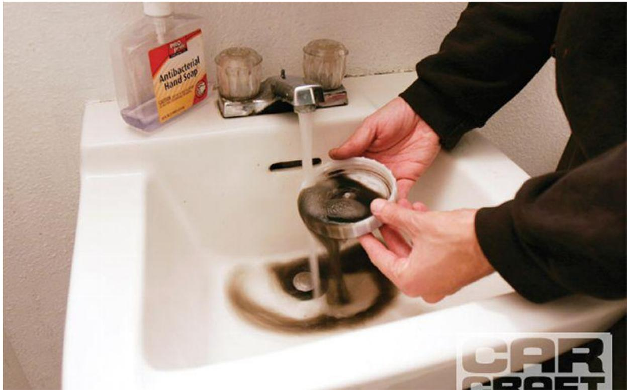
Proving that this is really waterborne paint, it cleaned up with nothing but pure water. If you are going to be doing this often, don't just pour the stuff down the drain. There is a recommended disposal procedure. As we mentioned earlier, we cleaned out the gun with rubbing alcohol rather than lacquer thinner.
