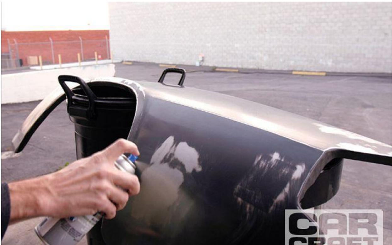
We found an abandoned Camaro quarter-panel lying out behind our shop, cleaned it up, and prepped it for paint. The e-coat primer was still in good shape except for a few spots where it had chipped off and rust had started to form. We removed the rust with a wire brush on an air drill rather than using a grinder because we wanted to remove as little metal as possible. Once the rust was gone, we sprayed all the bare steel with Dupli-Color etching primer we bought at our local parts store.
