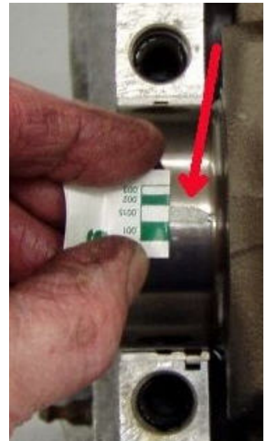
Bearing Clearance Measurement
