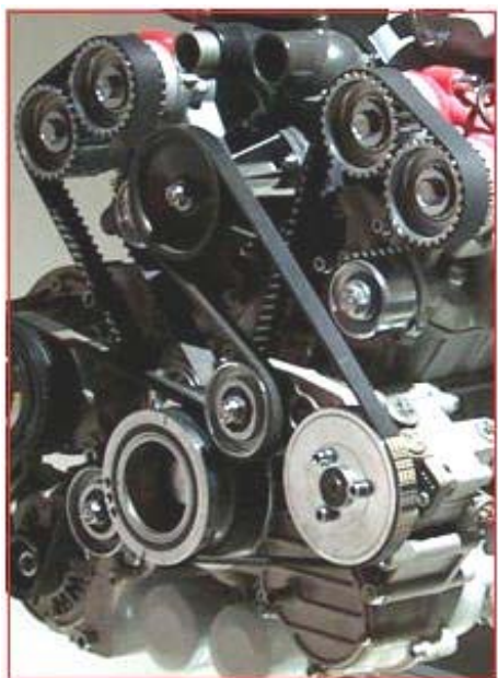
Belt drive, left; Gear drive, below
