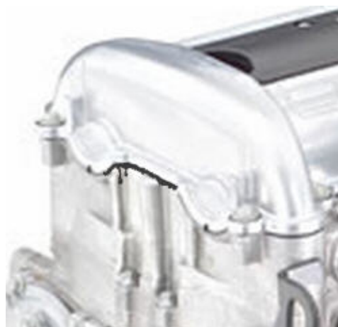
Using Foot Powder for Visual Leak Detection
