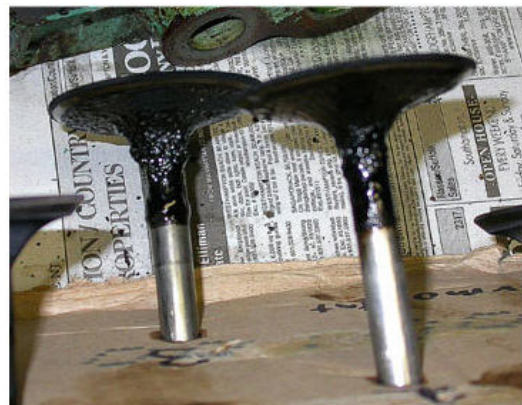
Carbon Deposits on Intake Valve
