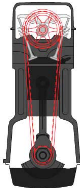
Timing Gears and Belt
