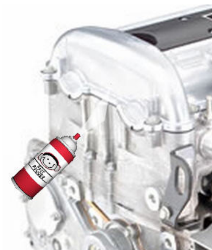
Using Foot Powder for Visual Leak Detection
