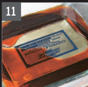
To begin etching, we placed our body tag in the acid face up, making sure to cover the plate with at least a 1/4-inch of solution.
