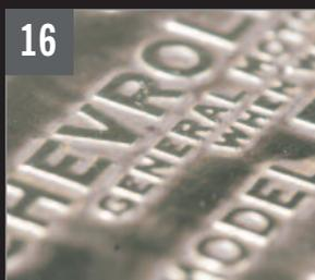
As you can see, the metal was etched evenly, leaving well defined letters intact with enough depth to fill in with paint.
