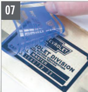
After quenching, we peeled the translucent backing away, completing the transfer of our body tag design to the brass.
