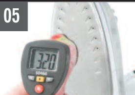
We used a household iron to apply the heat and pressure needed to transfer the design to the metal. Our goal was a temperature range of 275 to 325 degrees without steam.
