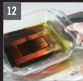
Because the metal will etch unevenly if left to soak, we agitated the solution every couple minutes. This also helps flush the areas being etched.
