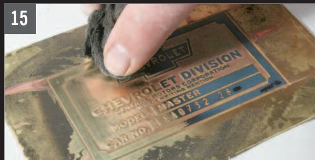
After rinsing the brass thoroughly, we peeled off the protective tape before using steel wool to remove the toner mask.
