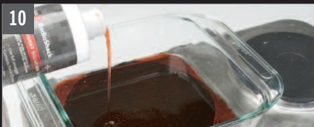
While ferric chloride etchant solution (available at Radio Shack for around \$10/bottle) will work fine at room temperature, we discovered it's more effective at about 120 degrees. Read the warning label carefully first and make sure to use it in a well-ventilated area while wearing rubber gloves and eye protection. Also, make sure to use a glass container opposed to a metal one, as the acid will not penetrate glass.
