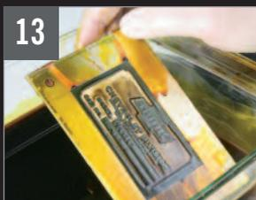
We checked the etching depth often, as the time needed varies with each metal. Our brass plate took about an hour to etch our desired amount.
