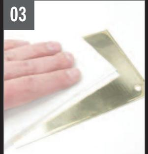
Since brass sheets are tough to come by, we elected to use a brass door kick plate and sanded off the clearcoat finish. Then we cleaned the surface with mineral spirits to remove any grease or finger prints.
