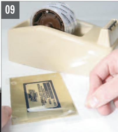
Before starting the etching process, we masked off the remaining exposed surfaces of the brass plate that we didn't want etched, including the back side. We used packing tape because it resists the effects of ferric chloride.
