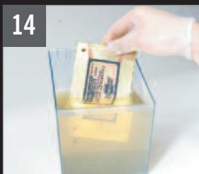
After removing the plate from the etchant solution, we neutralized it by soaking it in cool, clean water.
