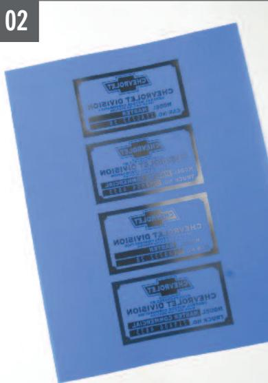
We used a laser printer to print our body tag design on the rough side of the PNP-Blue, purchased online for about \$1/sheet. After printing, we removed any lint or dust from its surface to ensure a proper transfer to the metal. If any particles remain when transferred, they will lead to imperfections in the form of pitting in the unetched portion of the metal.
