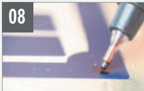
Small imperfections occurred where the toner didn't completely transfer to the metal. To fix this problem, we applied a couple layers of ink using a black Sharpie marker. We used black finger nail polish for fixing larger exposed areas.
