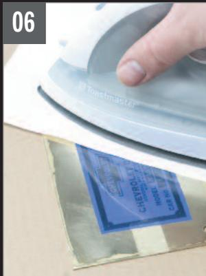
Using a piece of plain white paper to reduce friction, we made smooth passes over the transfer making sure to apply even heat. After about five minutes, we brought the temperature of our brass plate to the 275 to 325-degree range. After transferring the design, we quenched the metal in cold water. Quenching allows the toner mask to adhere solidly to the metal.
