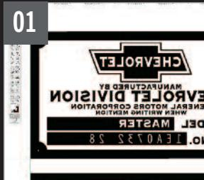
The first step in the process is creating a design. The black areas in the design will mask the metal and the white areas will be exposed to be etched. In order for the design to turn out correct, it must be reversed before being printed and transferred.
