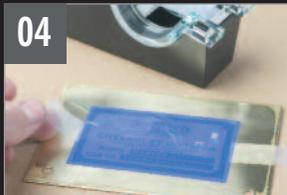
Before transferring the design to the metal, we attached the substrate with removable tape to ensure the PNP-Blue didn't shift during transfer, which would compromise the mask.
