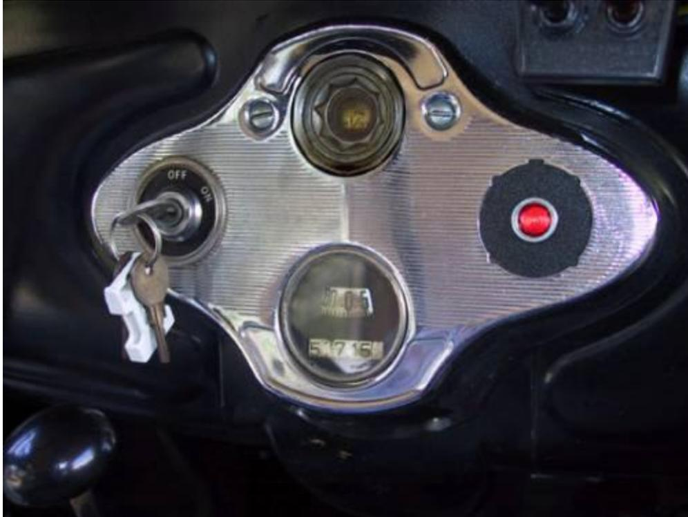
At the dash of the old Model A, the 15 AMP gauge was removed in favor of a Warning Light, which operates perfectly with the THREE-WIRE model 12SI alternator. (Shown with ignition ON, engine stopped.)
