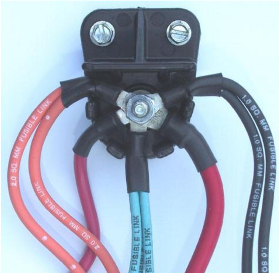
The insulated terminal block, is a sensible method of connecting a few wires together. It has a re-enforced shield above it to shed water, and separators between wires. It's a great little organizer in general. And it will be mounted remote from the battery, where it will stay free of corrosion.
