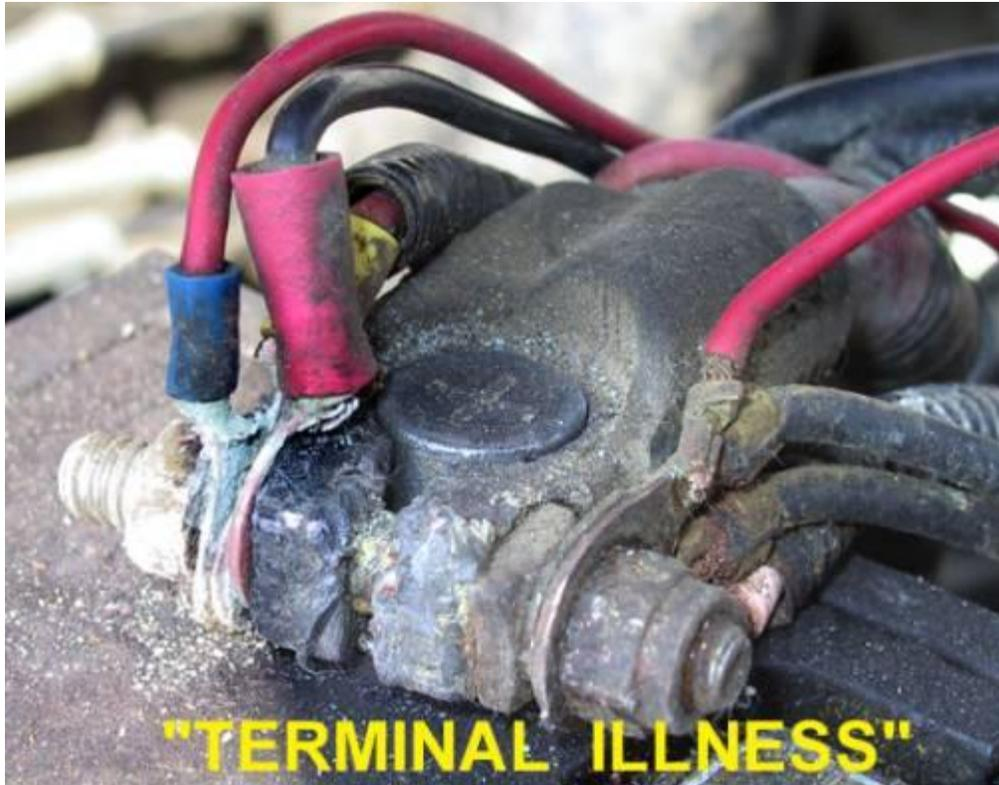
Okay, all these modern accessories that come with instructions to connect a wire directly to the battery POS, and the instruction to connect a cable from the ONE-WIRE directly to the battery, has resulted with a clutter at the battery area. And thanks to the 100 amp ONE-WIRE alternator (a high rate battery charger indeed), the wires are a corroded, unreliable, mess!
