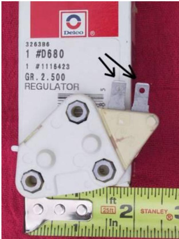
The difference between the ONE-WIRE and THREE-WIRE alternator is the **voltage regulator**. The Delco part # D680 voltage regulator shown above is used in both the 10SI and 12SI THREE-WIRE models. The same model of alternator can be assembled with different types of voltage regulators (for ONE-WIRE or for the THREE-WIRE system). We do have options, and the choice is ours to make.
