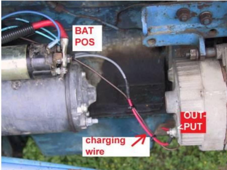
And the **wire harness** on tractors and most other machinery **is short in length**, with fairly heavy gauge size wire. The ONE-WIRE alternator could satisfy the battery charging needs on this simple old tractor.
