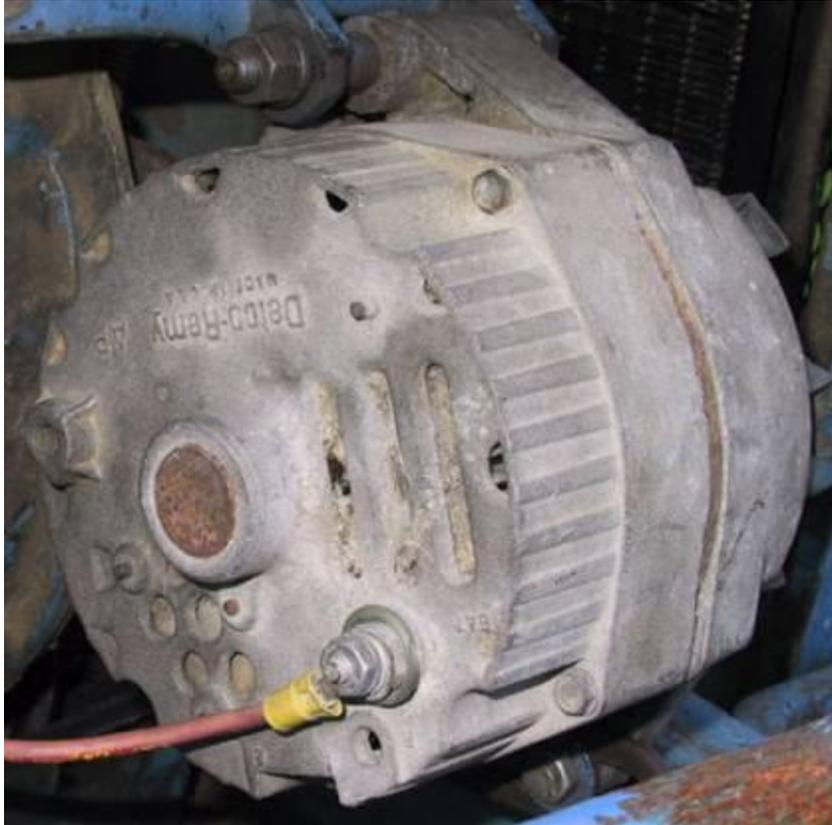
**Shown above** is the first-generation GM Delco-Remy alternator with built-in voltage regulator. The "ONE-WIRE" alternator shown above only has a heavy gauge wire connected from the output terminal to the battery. The obvious advantage is that not much knowledge is needed to wire it! (The ONE-WIRE alternator shown above is the 10SI model.)
