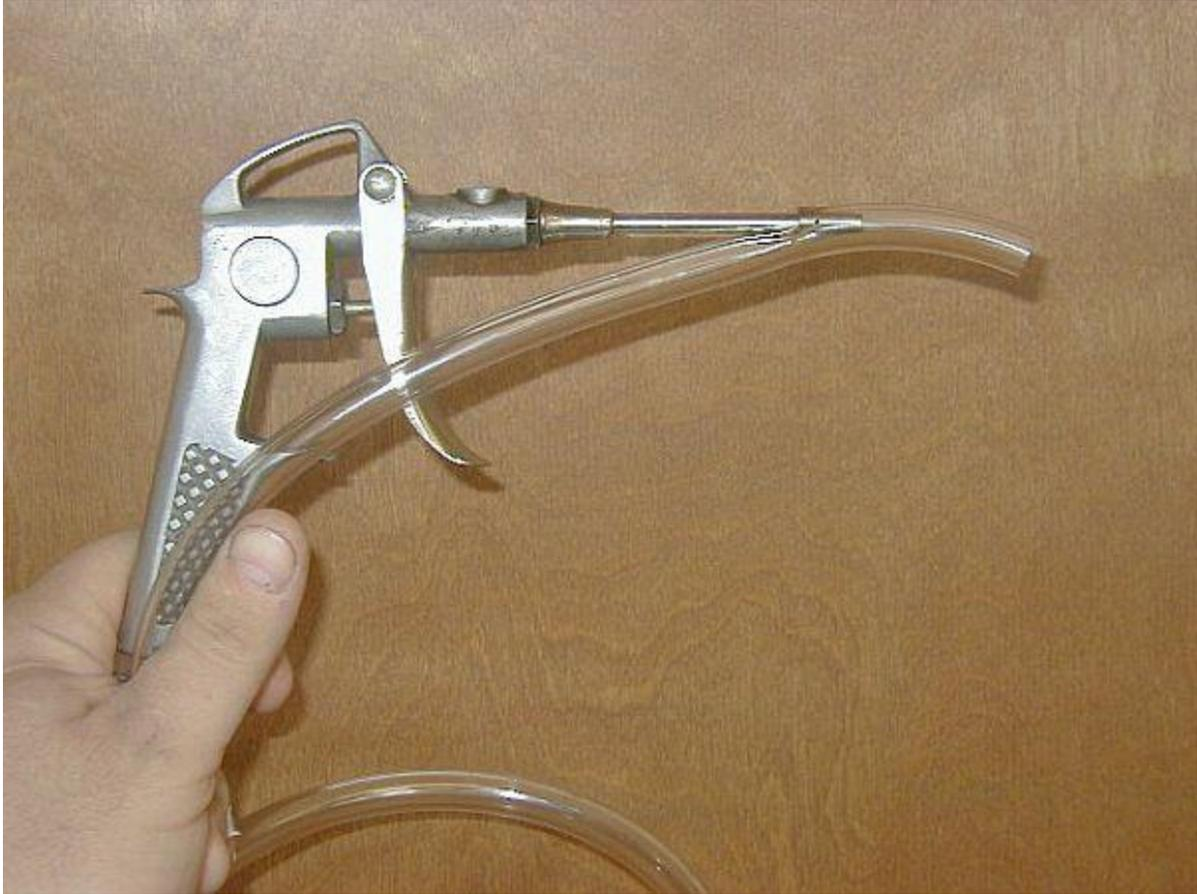
Positioning your wand tip like this will create a venturi effect in the hose causing the soda to be pulled up from the box by low pressure and mixed with the high pressure air from the wand. Use one length of tape to wrap around the end of the air wand and hose. This will keep the hose in the proper position on the wand tip during blasting.
