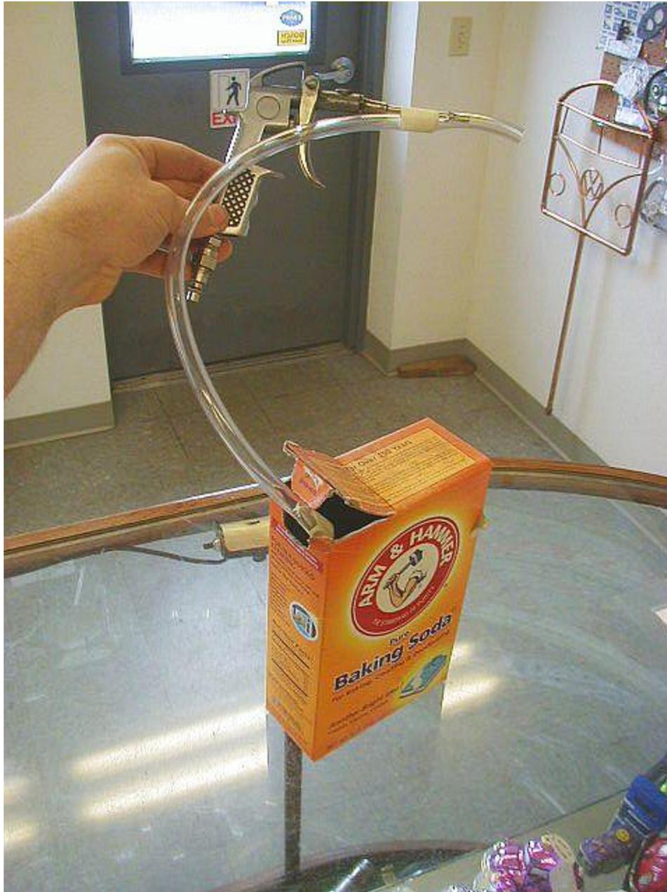
**WARNING: Blasting should ONLY be done outside in a well ventilated area such as a patio or concrete driveway. Of course proper eye protection and a face mask should always be worn. Baking soda is not poisonous but it feels like your breathing a soft drink if you inhale it and it's irritating, so protect those lungs!!**
