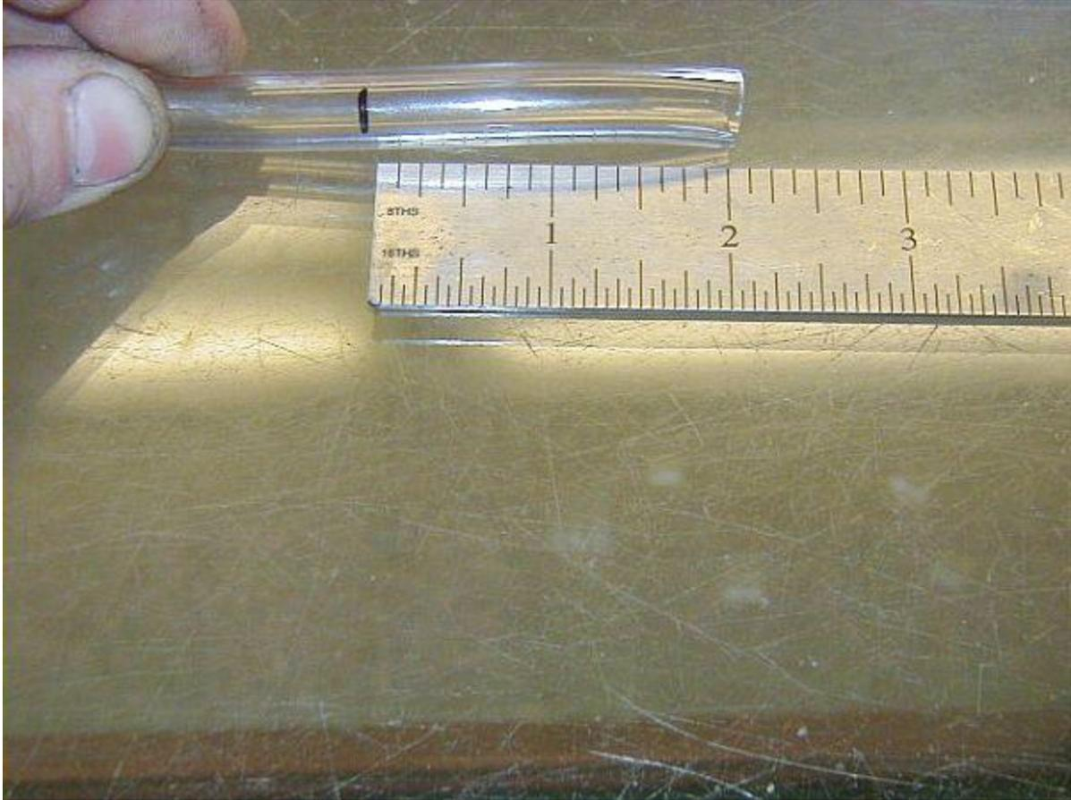
Take your knife or razor blade and make a small cut across the hose **ONLY** through one side. The cut needs to be just large enough so that the tip of the air wand attachment will stick into the hose. Stick the tip of the air wand into the hose and let it stick in about 1/4" - 1/2".
