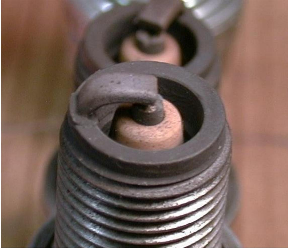
**Shiny or Glazed Porcelain:** This occurs for two reasons, excessive idling or rich idle condition leaving heavy soot deposits. These deposits will burn and create excessive porcelain temps causing the glass to melt usually resulting in a down track popping through the exhaust..
