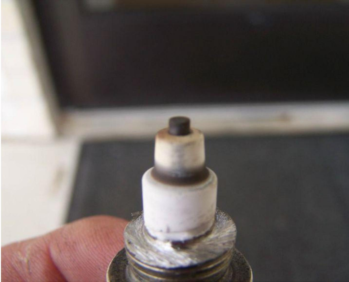
**Shiny little diamond like deposits:** It's too late you've already started to blow the pistons out of it. Start over from scratch, fatten the carb, back-up the timing and cool down the plugs. Now start a proper tuning procedure and hopefully you caught it before too much damage was done.
