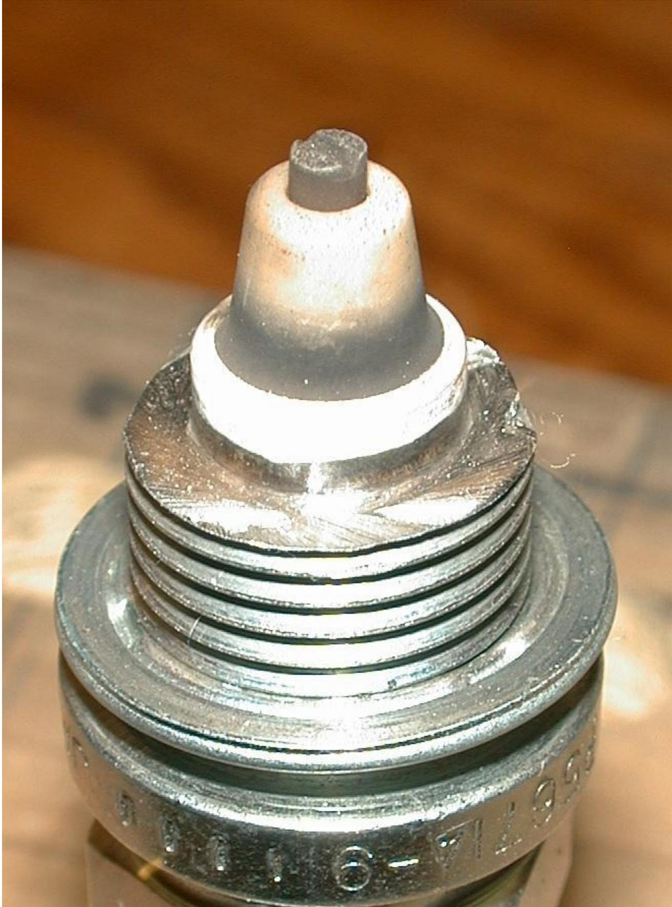
**Black or brown specs:** This is an indication of detonation usually caused by too hot of a plug, drop one or two heat ranges and it should go away.
