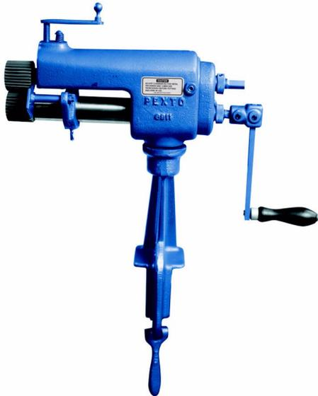
A combination Rotary Machine embodying all the features of the Throatless Machine with the added features of a 7" throat, and arbors designed to utilize crimping, beading, furnace collar edging and offset rolls. See Roll Chart for rolls available.
