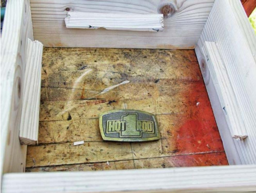
05] We got 5 gallons of casting sand from Alcast, a local foundry that casts everything from fuel nozzles to Ford Boss 429 heads. You can make your own casting sand, but we wanted to remove as many variables as possible. The sand is fine and contains binders and water that make it just a bit sticky. You know the sand is the right consistency when it keeps its shape after being formed by hand.
