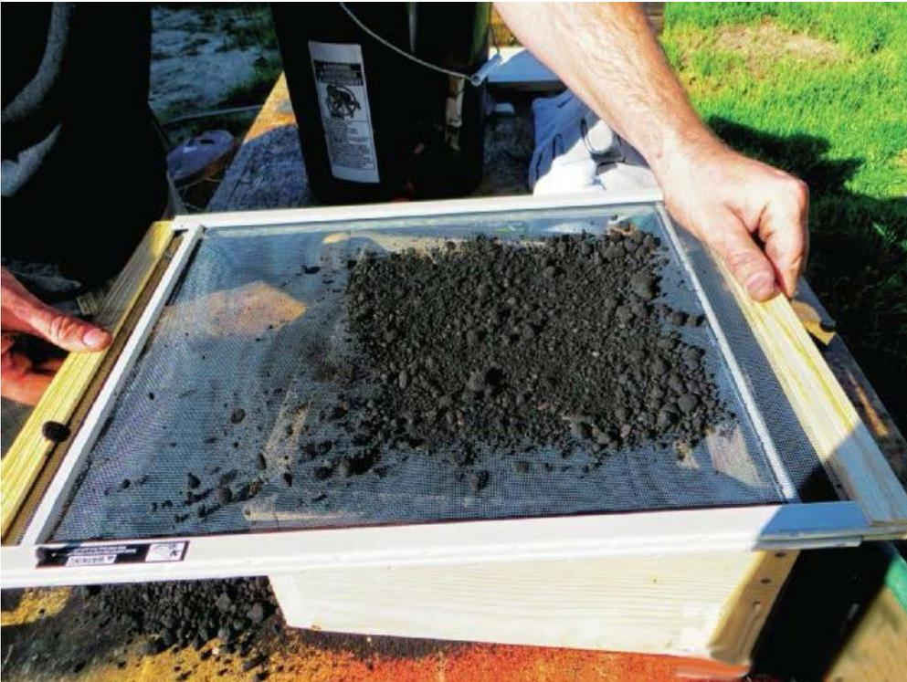
07] We sifted several inches of sand onto our pattern before we used a two-by-four to compact the sand all around the pattern. Sifting is only needed on the sand near the pattern, so we simply compacted scoops of sand until the flask was full.
