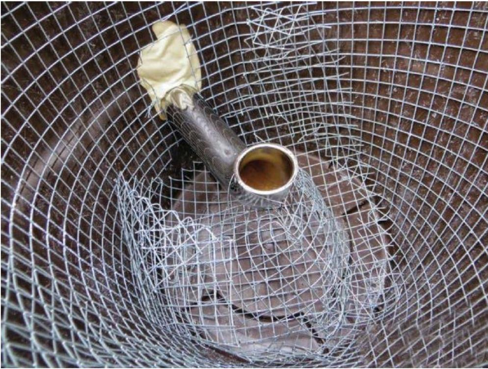
03] The mixed concrete was poured into the plastic planter until it met the drain. We packed some of the wet concrete into the hardware cloth before we dropped in the terra-cotta and packed concrete around it. We gave it four days to set.
