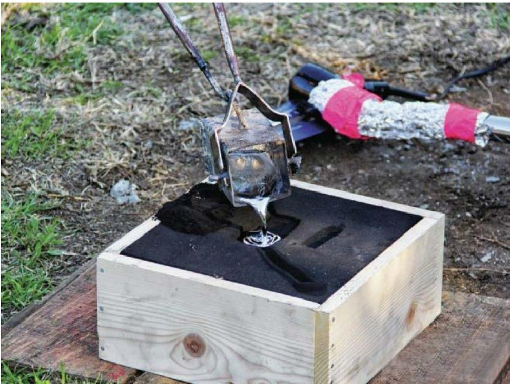
15] An empty aluminum can set in sand in our second flask served as a mold for an ingot of
