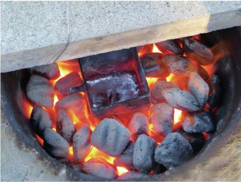
14] The crucible we built from square tubing has two pins on the side that allowed us to use a forked tool to lift it out and a hook to tilt it. Not as elegant as tongs, but they worked, and the aluminum poured out easily.
