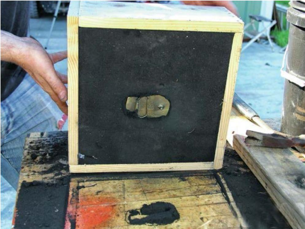
09] A couple of taps to the back of the belt-buckle pattern ensured it was loose before we pulled it free. The center of the mold was clean, so we just blew the loose sand from the
