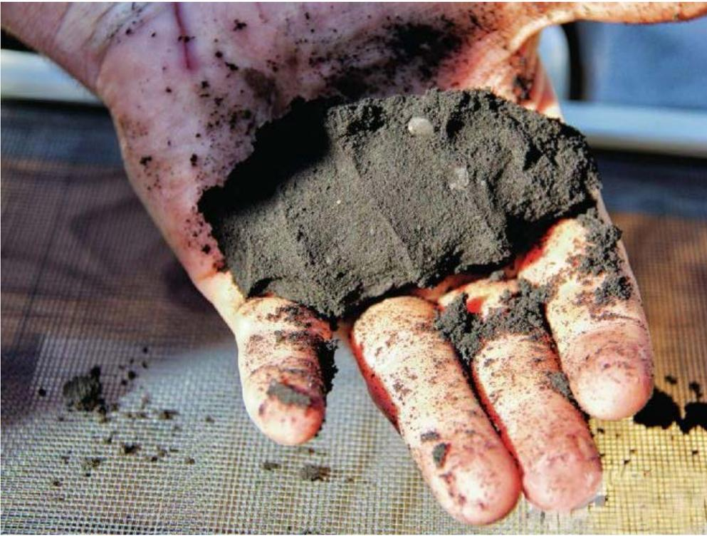
06] A \$7 window screen was used to sift sand over the pattern. Sifting keeps fine sand near the pattern for a more detailed, smooth casting. You can see the clumps of sand that didn't get through the mesh.
