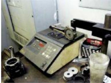
Here, the small end of the rod is being weighed to help determine the reciprocating weight.
