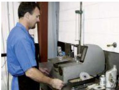
Earl Mark of Automotive Specialists checks each half of a bob weight individually to make sure that the total weight is correct, but also that both sides of the bob weight are equal.
