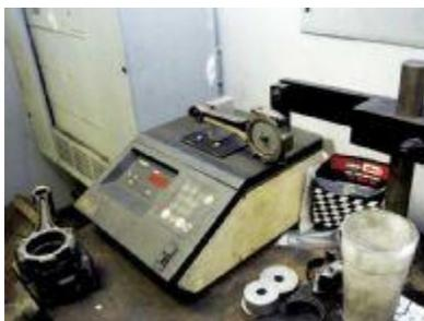
Here, the small end of the rod is being weighed to help determine the reciprocating weight. As you can see, the rod is assembled when it is weighed. A stationary arm suspends the end that isn't being weighed over the scale.
