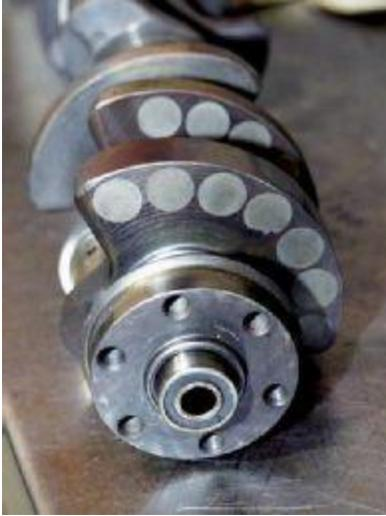
This crank is essentially junk, but you can see the many slugs of malleable metal that have been
