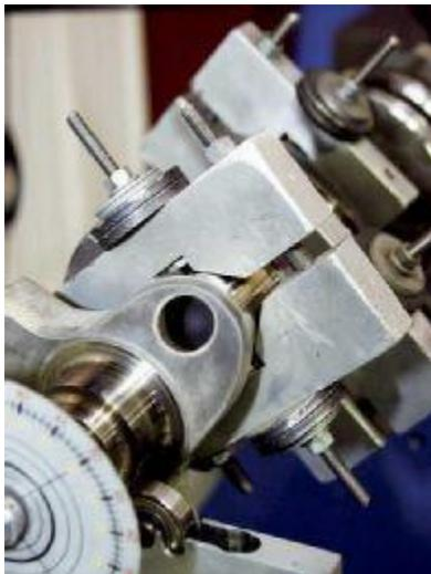
Bob weights, which simulate the weight and motion of two rods, two pistons and the rest of
