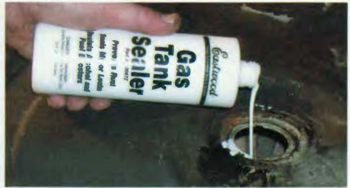
Gas tank sealer prevents future rust and seals minor leaks. It's also resistant to alcohol.
