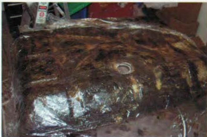
Paint stripper is used to remove the paint on top of the tank. Plastic prevents the stripper from evaporating before doing its job.
