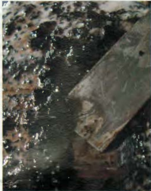
Use a putty knife and "Undergone" to remove undercoating. This is a messy job, so have plenty of old newspapers covering the floor.
