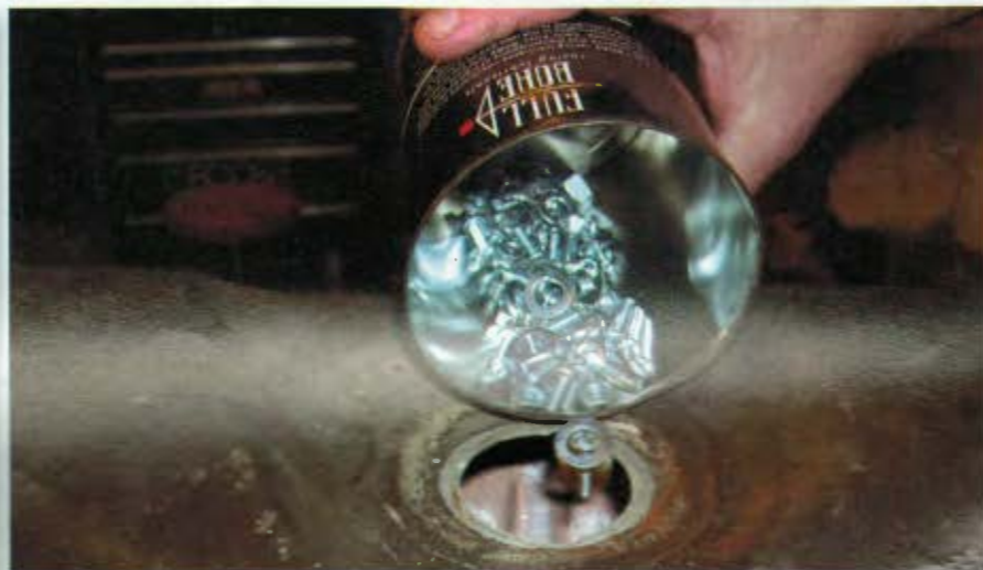
Nuts and bolts dumped in to the tank help loosen rust and scale.
