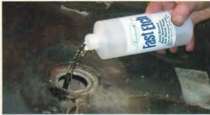
Eastwood's "Fast Etch" removes rust and etches the metal. It's part of their gas tank resto kit.
