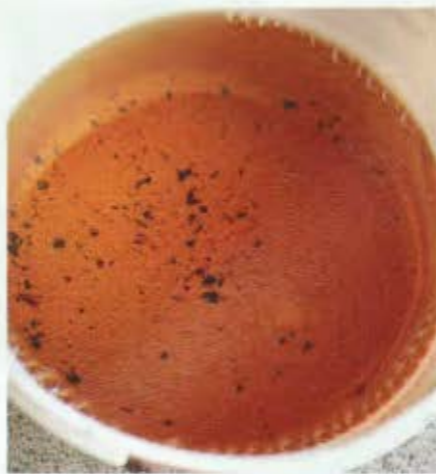
Sample of the remaining gasoline indicates loose rust and scale.
